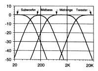
The Quad-amp system takes maximum advantage of the modules' cascading capability. This system uses no passive crossovers, and each driver has a dedicated amplifier.
