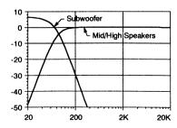
This system is identical to the SWX Bi-Amp System, except that the EQM module is added for extra bass boost.
