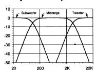
For 3-way systems without dedicated midbass drivers this system provides very good response. The 24dB/octave slopes allow midrange drivers to be safely crossed over at lower frequencies than they can be with 6 or 12 dB/octave slopes.
