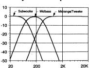
This system shows how the SWX and MRX modules can be used together. Note how the 24 db/octave slopes precisely define the frequency band of the midbass driver.
