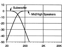
In this system, the SWX crossover module is used to divide the music between a mono subwoofer and stereo midrange/tweeter satellites. The KICKER amp's self-bridging feature is used to drive a mono subwoofer from a stereo signal. Passive crossovers are still needed for the midranges and tweeters.
